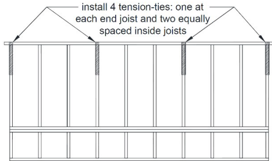
FIGURE 18 - TENSION TIE LOCATIONS
