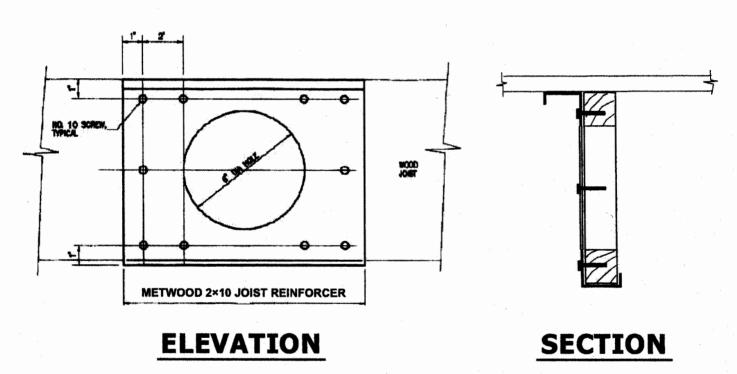
10 fasteners shall be used in the predrilled holes located as indicated above. The fasteners shall be  $1^{1}/_{a}$ -inch-long No. 10 wood screws.
